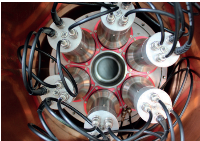
Compton suppression ring, comprised of NaI detectors, surrounding a high-purity germanium detector
